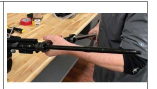
NOTE: The barrel nut does not need to be indexed, so over torquing is not necessary.
